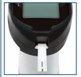
2. Remove test strip from vial and close vial immediately. Insert strip into Test Port with black blocks facing up. The meter turns on.
